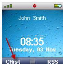
The CHist button offers three options: Missed, Received, and Dialed calls (image A). Each option will present a list of contacts (image B). Once a contact has been selected, more options are presented: Detail, Delete, and Save to directory (image C). Once Detail has been selected, the contact's name and number and date/time are presented (image D).
