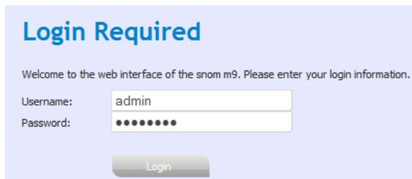
**Important:** The device will be inaccessible if both the DECT PIN and the Web portal password of the snom m9 are forgotten. Under these circumstances, the base station can be reverted back to factory default by dialing the recovery code `**0000**` from any registered handset.
