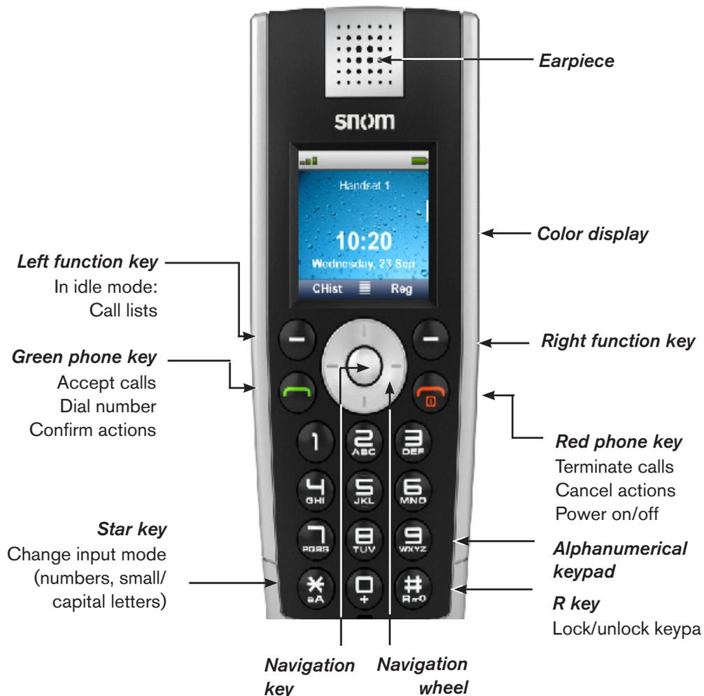
**Navigation key:** In idle mode, press the center navigation key to get to the main menu. In other contexts, press this key to navigate the menus and lists.
